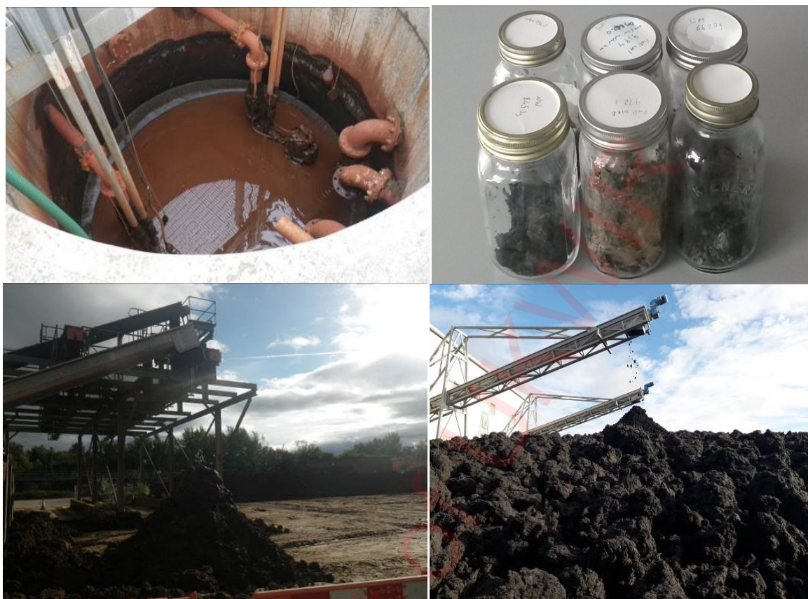
Figure 3 Liquid sludge at LRS1 WTW, various sludge samples dried in jars with air permeable glass fibre filter lids, solid sludge at LR2 WTW and AAD1a WwTW.
