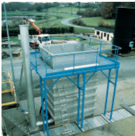
The new Degremont-Pulsator unit for training on the operation of settling tanks using thin sludge layers
