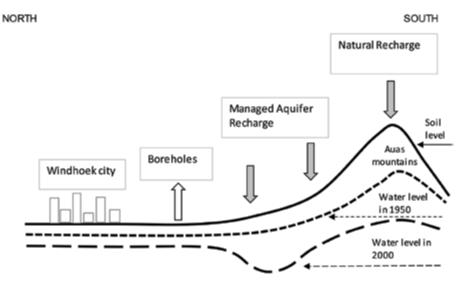
Figure 3: Scheme of the managed aquifer recharge in Windhoek (adapted from Mathews, 2003).
