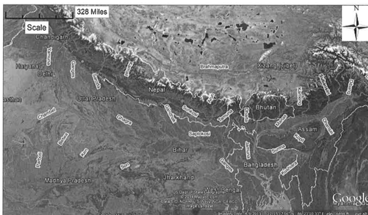
Figure 4 Digitized river network for the entire GBM basins used in HEC-RAS river model.
