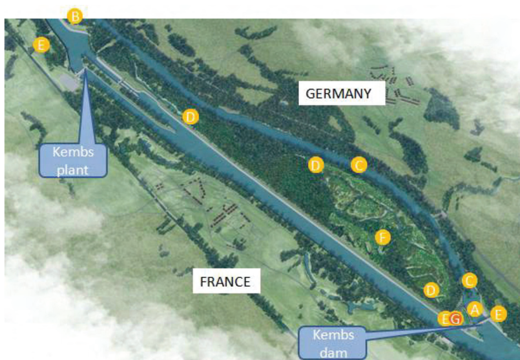
Figure 2: Location of the main environmental measures : ecological flow (A), “controlled erosion” (B, and other locations further north), injection of gravels (C), fish and aquatic mammals connection (E), recovery of wetlands (F) and new hydropower plant (G). (Artist view).
