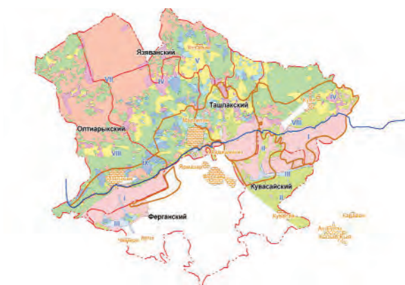
Figure 14. Updated hydro-module zoning for five districts in the Fergana province of Uzbekistan (The different colours show areas with different soil fertilities and levels of groundwater)
