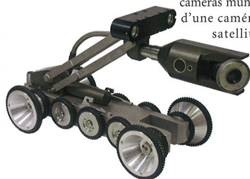
Caméra HV 180 TO 100 phare (Hydrovideo).
