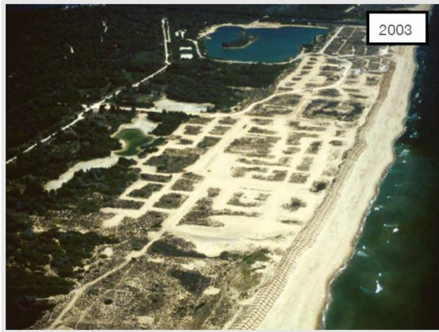
2003: During the LIFE DUNA project: Malladeta north and Brava beaches. The boardwalk has been removed and replaced by a dune system/cord. This has been set back 5m inland with respect to the boardwalk. The roads and car parks have been eliminated.
